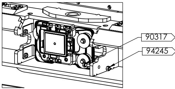
TORQUE TO 6 FT-LBS (LUBRICATED) / 8 FT-LBS (DRY). REPEAT FOR OTHER SIDE OF TRUCK.
