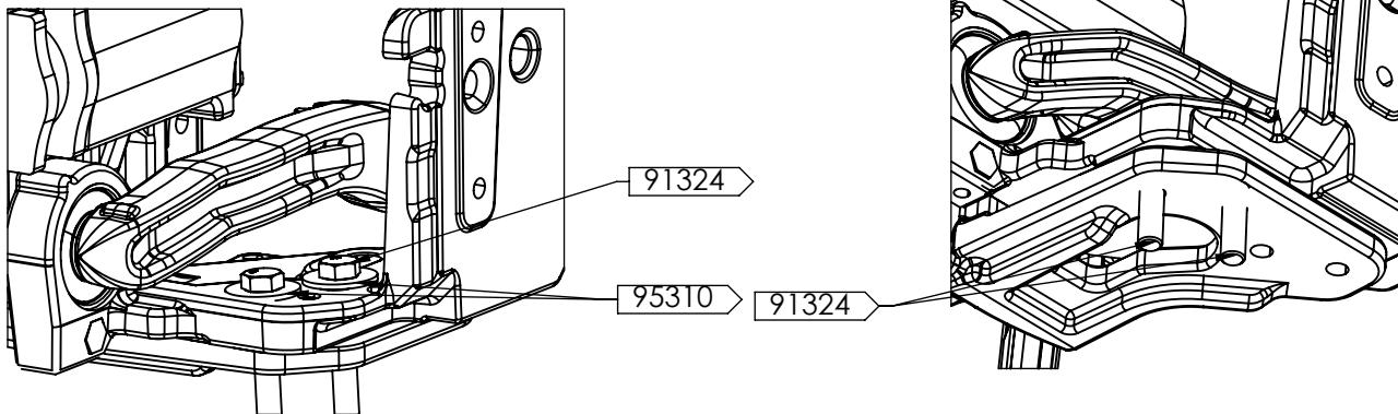
8. ATTACH THE MOUNT BRACKET (**65616**) TO THE DRIVER SIDE OF THE TRUCK AND MOUNT BRACKET MIRROR (**65616M**) TO THE PASSENGER SIDE OF THE TRUCK. SECURE THE BRACKETS USING THE FOLLOWING HARDWARE:
