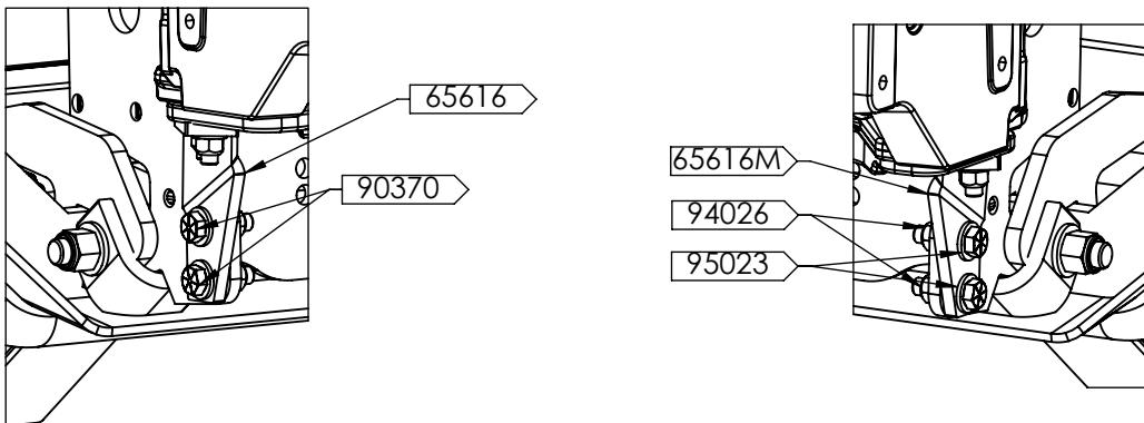
14. ATTACH THE FOG LIGHTS TO THE GUARD WITH THE FOLLOWING HARDWARE:
