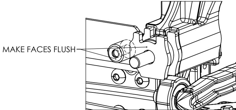
11. SECURE THE TOW MOUNT ASSEMBLY WITH THE FOLLOWING HARDWARE:
