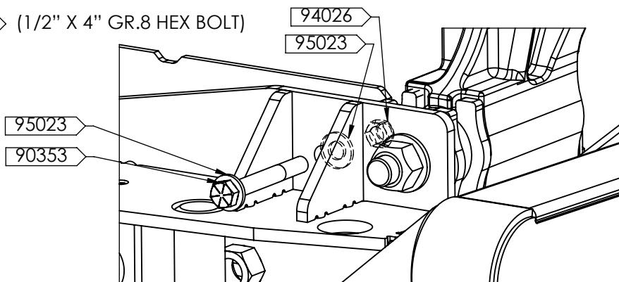
TORQUE TO 53 FT-LBS (LUBRICATED) / 107 FT-LBS (DRY). REPEAT FOR OTHER SIDE OF TRUCK.
