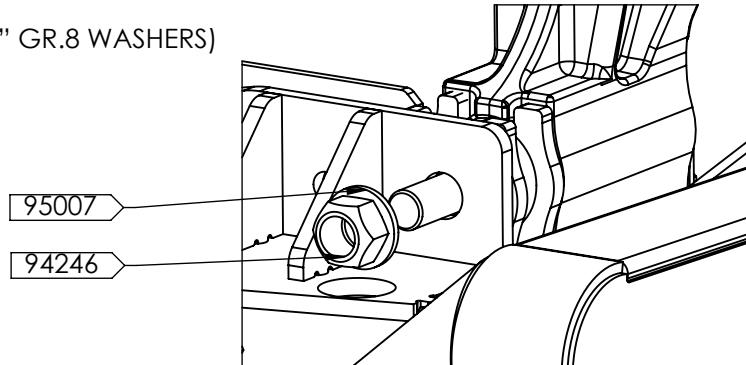
TORQUE TO 160 FT-LBS (LUBRICATED) / 210 FT-LBS (DRY). REPEAT FOR OTHER SIDE OF TRUCK.
