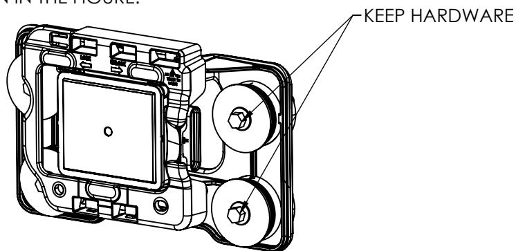
3. REMOVE THE FOLLOWING SCREW AND NUT FROM BOTH SIDES OF THE TRUCK.
