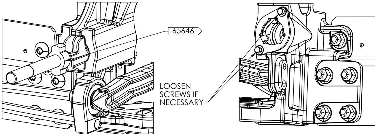
5. INSERT THE TOW RECEIVER SPACER WELDMENT (65614) OVER THE TOW MOUNT ASSEMBLY (65646) UNTIL IT CONTACTS THE FRONT FACE OF THE TOW RECEIVER. REPEAT FOR OTHER SIDE OF TRUCK.
