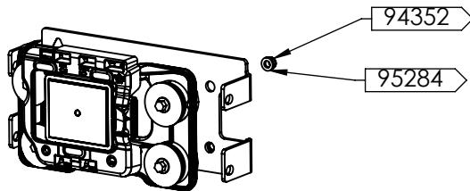
17. SECURE THE RADAR PLATE ASSEMBLY TO THE GUARD USING THE FOLLOWING HARDWARE:
