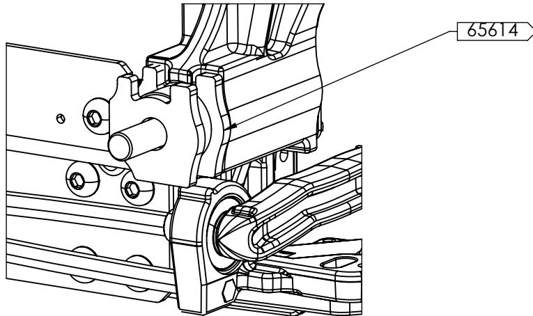
6. REMOVE THE TWO BOLTS IN THE LOCATIONS SHOWN BELOW ON BOTH SIDES OF THE TRUCK. KEEP THE OTHER TWO BOLTS IN PLACE.
