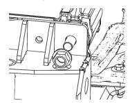
TORQUE TO 160 FT-LBS (LUBRICATED) / 210 FT-LBS (DRY). REPEAT FOR OTHER SIDE OF TRUCK.
