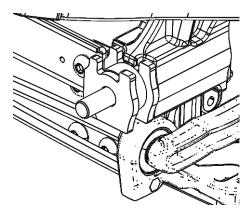
6. REMOVE THE TWO BOLTS IN THE LOCATIONS SHOWN BELOW ON BOTH SIDES OF THE TRUCK. KEEP THE OTHER TWO BOLTS IN PLACE.
