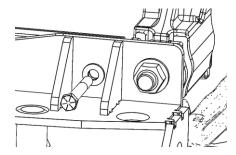
TORQUE TO 53 FT-LBS (LUBRICATED) / 107 FT-LBS (DRY). REPEAT FOR OTHER SIDE OF TRUCK.
