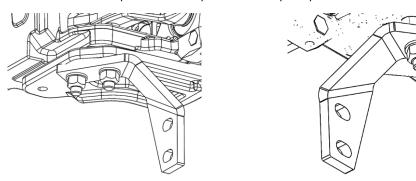
9. POSITION THE SPACER PIPE (65641) IN FRONT OF THE FRAME WHERE THE SCREWS WERE REMOVED IN STEP 3.
