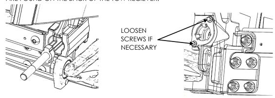
INSERT THE TOW RECEIVER SPACER WELDMENT (65614) OVER THE TOW MOUNT ASSEMBLY (65646) UNTIL IT CONTACTS THE FRONT FACE OF THE TOW RECEIVER. REPEAT FOR OTHER SIDE OF TRUCK.
