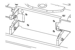
TORQUE TO 6 FT-LBS (LUBRICATED) / 8 FT-LBS (DRY). REPEAT THE PROCEDURE ON THE OTHER SIDE OF TRUCK. IF THE VEHICLE IS NOT EQUIPED WITH RADAR, THE RADAR PLATE MAY BE REMOVED TO ALLOW ACCESS TO THE CENTER TOW BAR.
