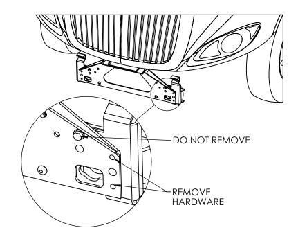
3. IF RADAR IS EQUIPPED ON THE TRUCK IT MUST BE REMOVED FIRST BEFORE INSTALLING THE MOOSE GUARD. KEEP THE ORIGINAL MOUNTING HARDWARE SEEN IN THE FIGURE TO THE RIGHT:
