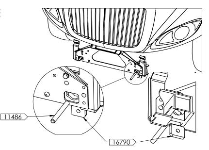
5. INSTALL (16769) ON THE DRIVER SIDE AND (16769M) ON THE PASSENGER SIDE. INSERT THE BRACKETS SO THAT (11486) GOES INTO ONE OF THE TWO BOTTOM HOLES. DEPENDING ON THE TRUCK ENGINE SIZE, THERE ARE TWO POSSIBLE CONFIGURATIONS, PLEASE SEE THE FIGURE ON THE RIGHT TO SELECT THE CORRECT HOLE.
