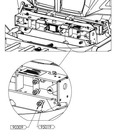
10. INSTALL THE FOG LIGHTS INTO THE GUARD. SECURE THE FOG LIGHTS USING THE FOLLOWING HARDWARE:
