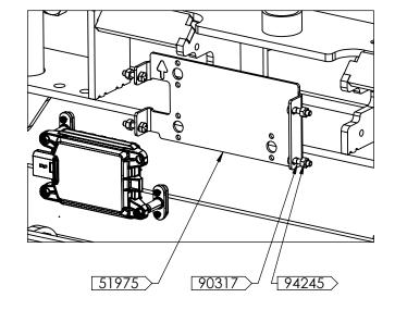
12. RECONNECT THE RADAR TO THE TRUCK (USE BRACKET SLOT TO FISH RADAR CABLE)
