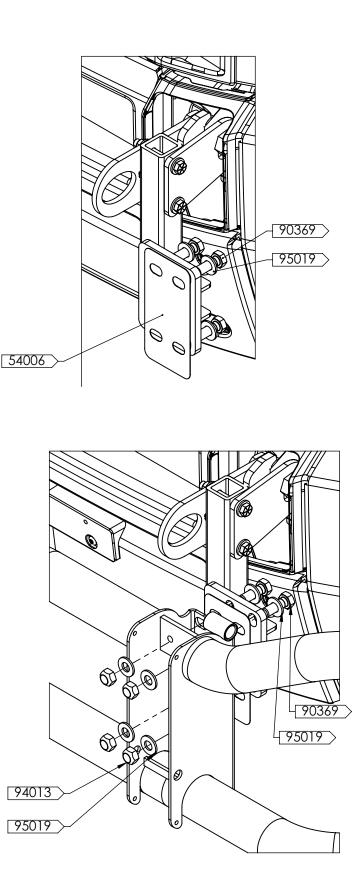
6. ATTACH THE MG-100B TO THE MOUNTING BRACKETS USING THE TOP ROWS OF SLOTS ON THE GUARD. USE THE FOLLOWING HARDWARE TO ATTACH THE GUARD:
