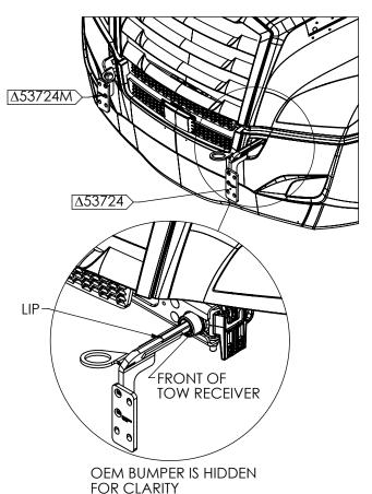
2. OPEN THE TRUCK HOOD AND INSTALL THE 34348 WASHER PLATE,
