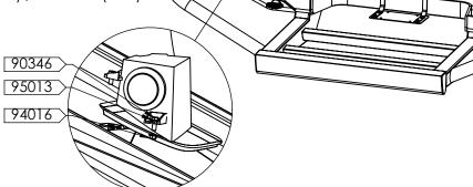
5. IF THE TRUCK IS EQUIPPED WITH RADAR INSTALL THE RADAR COVER ON THE MOUNT TABS OF THE BUMPER. IF NO RADAR IS EQUIPPED INSTALL THE ALUMINUM COVER PLATE 53296 . THE LICENCE PLATE CAN BE MOUNTED ON THIS PLATE USING THE ADDITIONAL HOLES. ATTACH EITHER OF THE COMPONENTS USING THE FOLLOWING HARDWARE:
