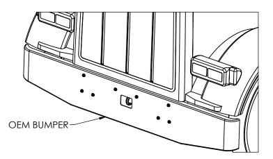
2. PLACE A STRAIGHT EDGE OVER THE TOW HOOK AND BUMPER MOUNT FACES. IF THE HOOK PROTRUDES FORWARD OF THE BUMPER MOUNT FACE, ADDITIONAL WASHERS WILL BE NEEDED AS SPACERS FOR BETWEEN THE TRUCK AND INSTALLED BUMPER.
