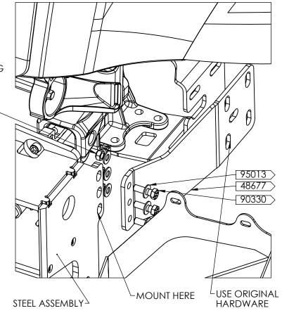
7. INSTALL THE FOG LIGHTS INTO THE BUMPER USING THE FOLLWING HARDWARE:
