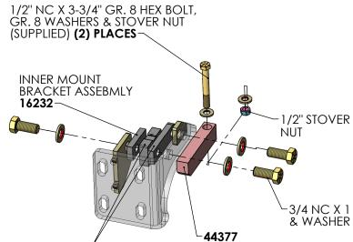
DETAIL B SCALE 1:7 -3/4 NC X 1 3/4" GR. 8 CAPSCREW & WASHER (SUPPLIED) (6) PLACES
