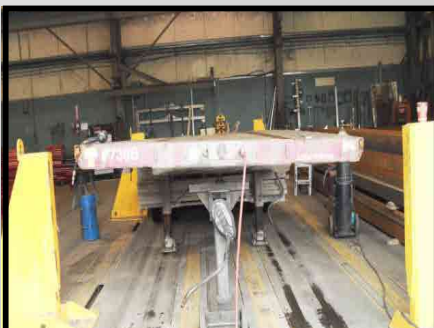
60' FRAME STRAIGHTENING BAY
